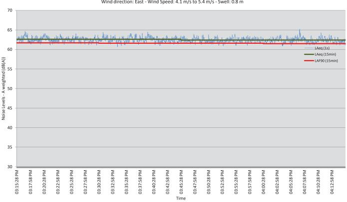
Pakiri Sand Extraction - Noise Level Measured at Position 2 - 07<sup>th</sup> May 2019 Wind direction: East - Wind Speed: 4.1 m/s to 5.4 m/s - Swell: 0.8 m
