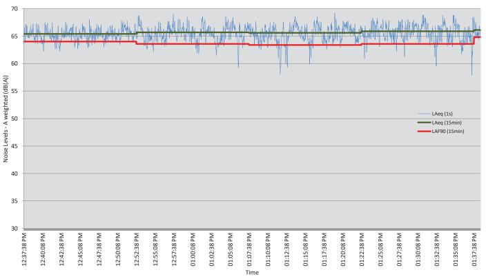
Pakiri Sand Extraction - Noise Level Measured at Position 6 - 11<sup>th</sup> July 2019 Wind direction: North - Wind Speed: under 1 m/s - Swell: 0.5 m Styles Grou Acoustics & Vibration Consultants
