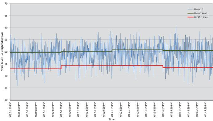
Pakiri Sand Extraction - Noise Level Measured at Position 6 - 22<sup>nd</sup> May 2019 Wind: Nil - Swell: 0.5 m
